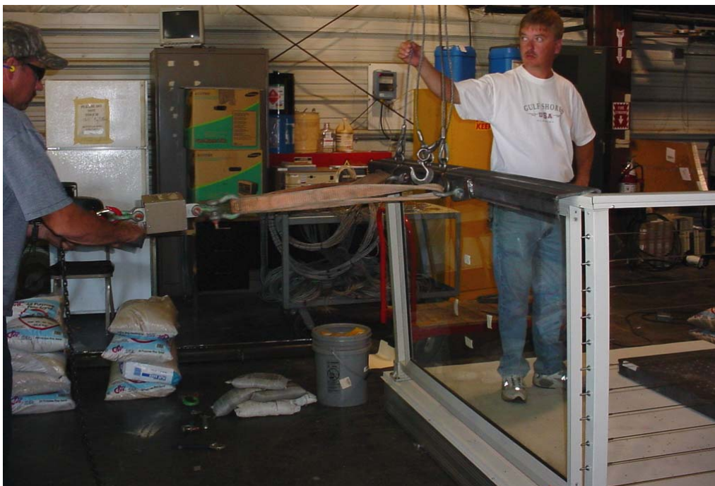
Photograph No. 6 Typical Horizontal Glass Side, Uniform Load Test
