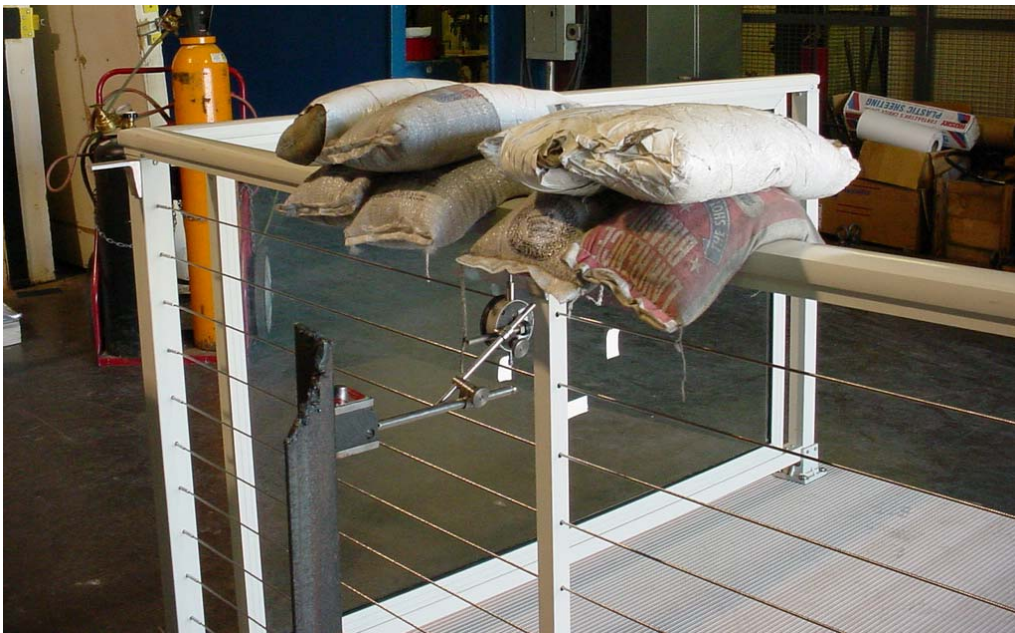
Photograph No. 8 Typical Wired Rail, Concentrated Load Test
