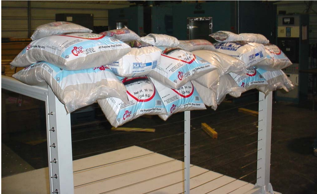
Photograph No. 5 Typical Vertical Wired Side, Uniform Load Test
