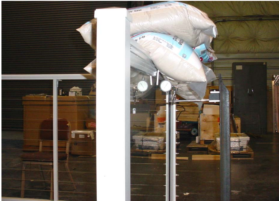
Photograph No. 10 Typical Glass Rail, Concentrated Load Test
