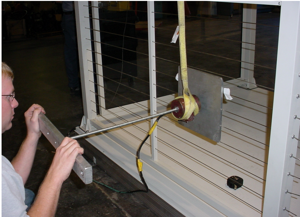
Photograph No. 1 Typical Center Wired Side, In-Fill Load Test
