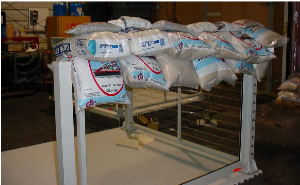
Photograph No. 4 Typical Vertical Glass Side, Uniform Load Test
