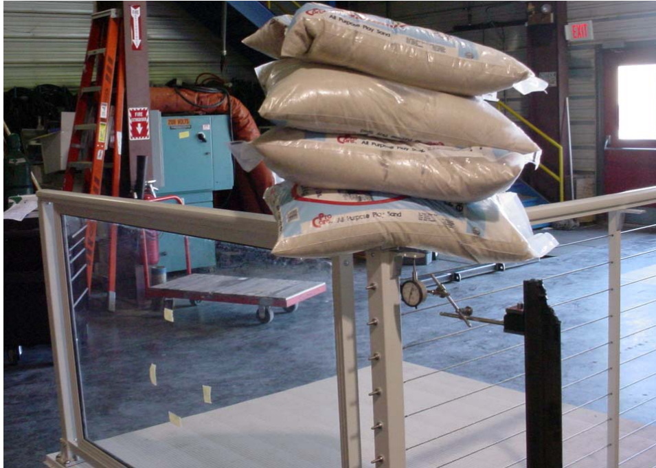
Photograph No. 9 Typical Corner, Post-Concentrated Load Test
