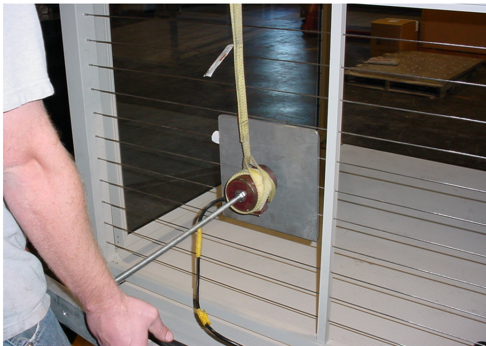
Photograph No. 2 Typical Near Center Post Wired Side, In-Fill Load Test
