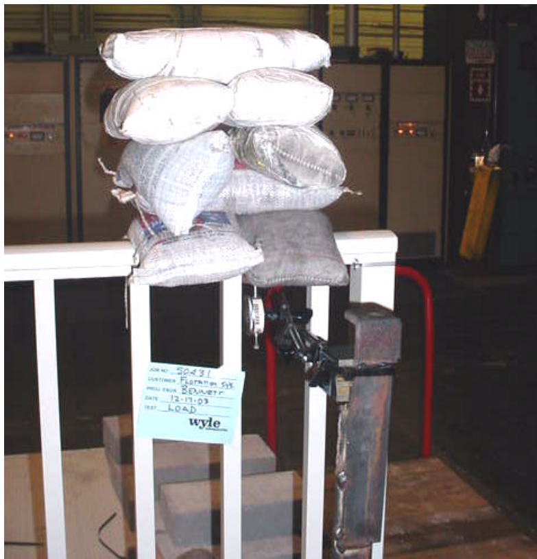
Photograph No. 4 Concentrated Load of 200 Pounds Applied in a Downward Direction
